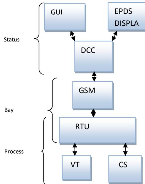
**Figure 4: Block diagram of distribution network remote monitoring system**
