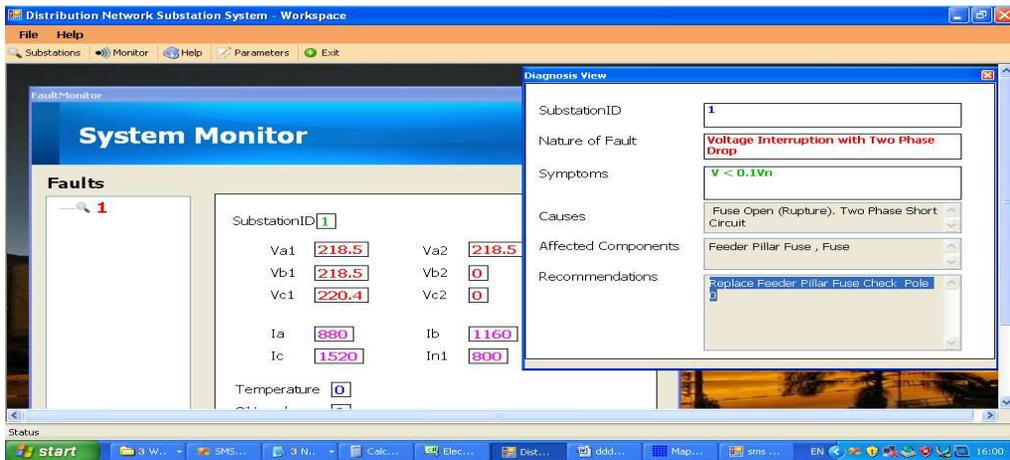
Figure 9: Voltage Interruption on two phases
