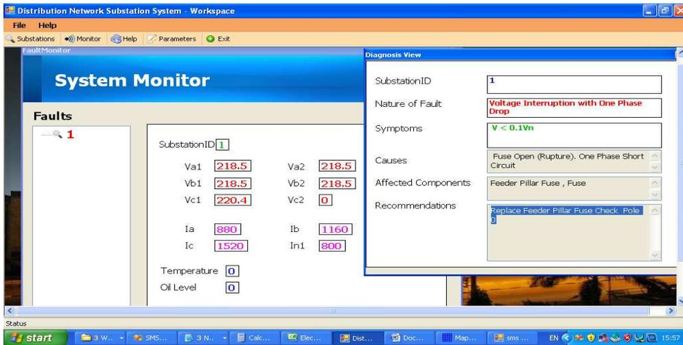
Figure 8: Interruption detection on one phase
