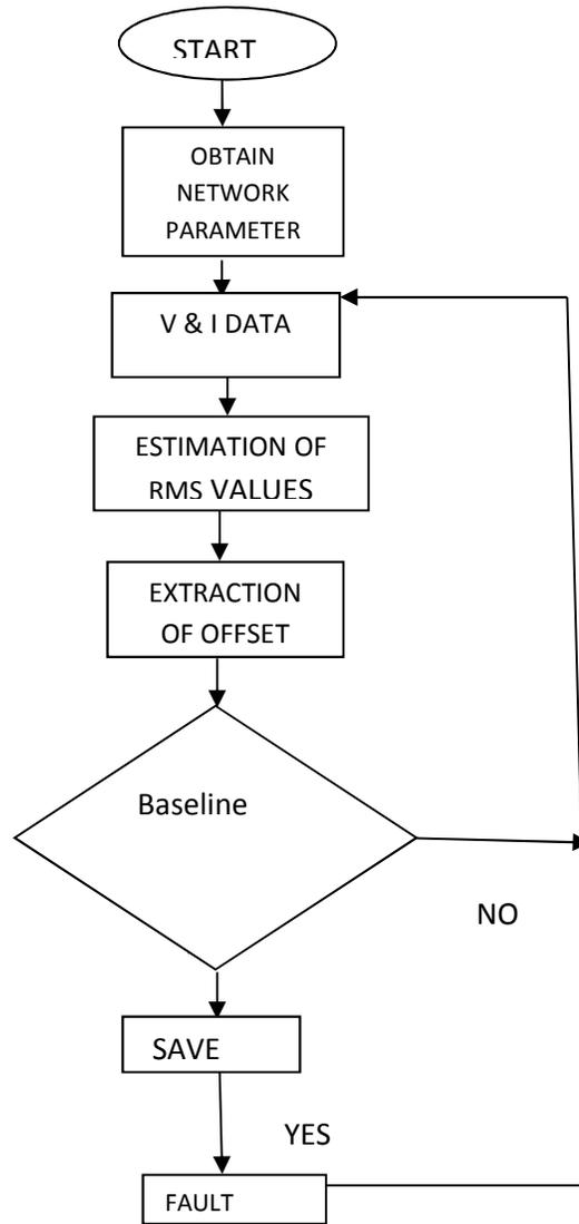
**Figure 3: Flow Chart for Outage Detection**
