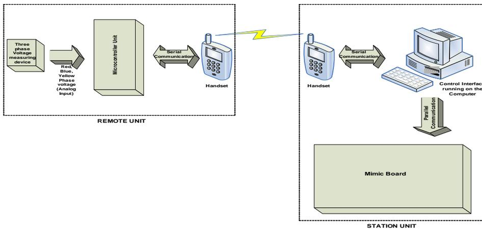
**Figure 5 Outage Detection Architecture**
