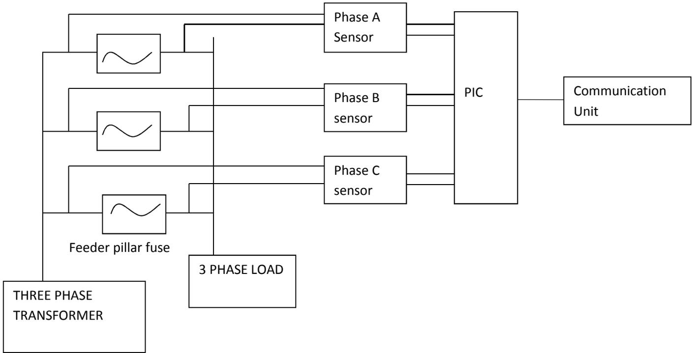
Figure 6: Block Diagram of Remote Terminal Unit
