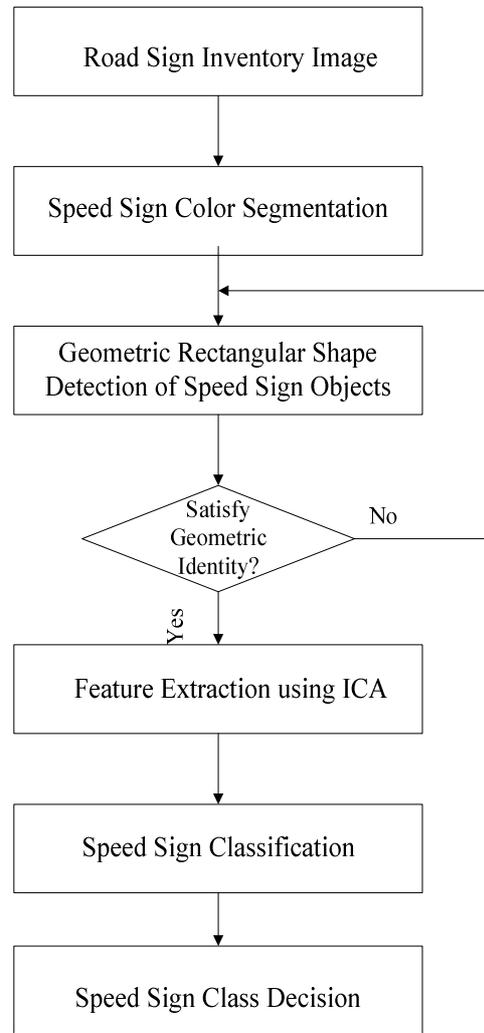
Fig.2. Flow diagram of the proposed system.
