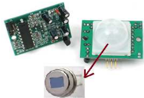
Fig. 4 A typical PIR sensor
